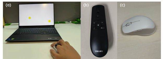
Figure 8: We built a Fitts’ Law usability testing system and used a touchpad and an airmouse as baselines. (a) The visualization interface and setup used in the experiment. (b) The airmouse used in the study. (c) The mouse used in the study.
