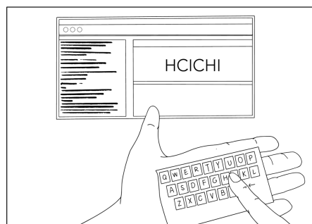
Figure 1: Demonstration of using the PalmPad system to input text directly in a VR scenario on the palm. (Left) A user interacts with his palm with finger taps, captured by a monocular RGB camera integrated into a head-mounted display. (Middle) The picture captured by the head-mount camera and the main feature of the finger used is amplified. (Right) An application scenario, where a virtual keyboard is displayed, allowing for text input via palm-based finger tapping.
