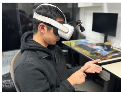
Figure 1: Demonstration of using the PalmPad system to input text directly in a VR scenario on the palm. (Left) A user interacts with his palm with finger taps, captured by a monocular RGB camera integrated into a head-mounted display. (Middle) The picture captured by the head-mount camera and the main feature of the finger used is amplified. (Right) An application scenario, where a virtual keyboard is displayed, allowing for text input via palm-based finger tapping.
