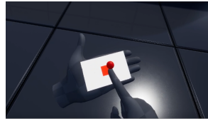
(b) MR interface display for the clicking experiment. Participants need to consecutively click on the position of the red square and report the number of errors based on the feedback provided by the system.
