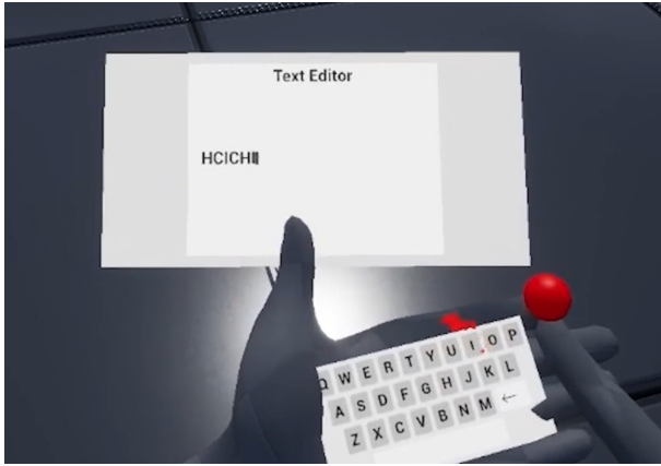
Figure 11: The keyboard application prototype supported by Palmpad in MR scene.
