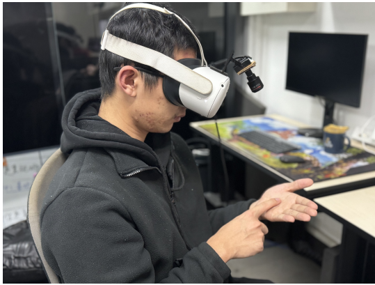
Figure 3: The hardware prototype and interaction method of Palmpad. A 120fps camera was fixed on the Quest 2 for input with an MR scene displayed through the Quest 2.
