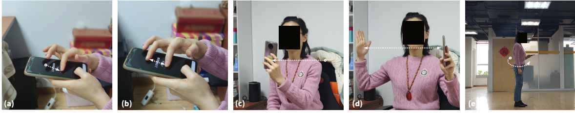
Fig. 11. A participant is using AngleSizer. (a) Using the one-finger gesture, with the right hand's index finger moving on the screen. (b) Using the two-finger gesture, to measure the distance between the right hand's index and middle fingers on the screen. (c) Using the one-hand gesture, to measure the distance moved by the left hand holding the phone. (d) Using the two-hand gesture. (e) Using the body-rotation gesture, holding the phone parallel to the ground and rotating by an angle.
