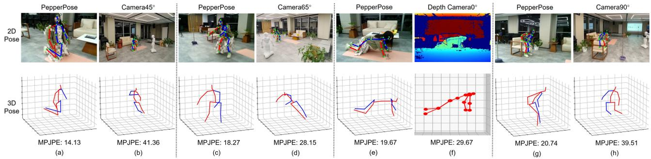
**Figure 9: Visualizations of the pose estimation results. Unlike PepperPose (a, c, e, and g) that can actively move and refine its viewpoint, stationary cameras are largely affected by unwanted orientations of the user (b, d, and f) and occlusions that caused by external objects in the environment (h).**
