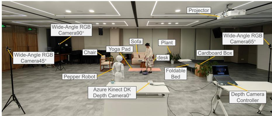
**Figure 7: The layout of our real-world experimental space. We put the essential equipment for actions apart from each other, as to help the participant to move and face diversely during the experiment, challenging the functioning of diverse pose estimation systems. The RGB and depth cameras are added as baseline methods for comparison.**
