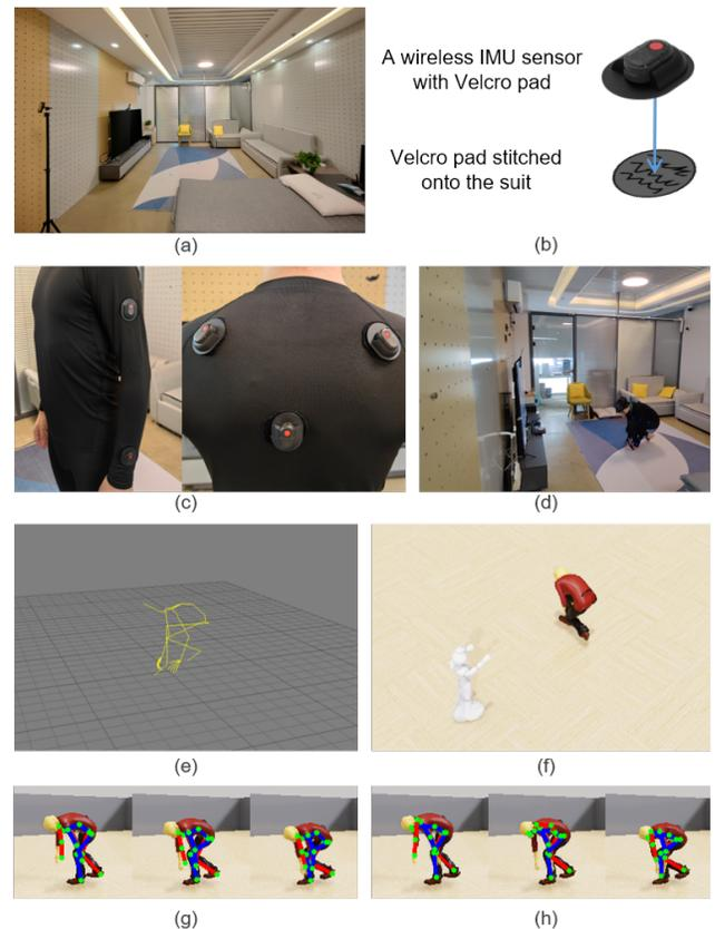
**Figure 4: To collect realistic data for training PepperPose, we (a) transformed the lab space into a home-like environment and (b-c) self-made comfortable suits with Velcro pads to accommodate the IMU sensors. (d-f) PepperPose is trained to interact with the people in Omniverse driven by such full-body 3D pose data. (g-h) By referring to the ground truth pose, the pose estimation module of PepperPose functions well on the simulated people.**
