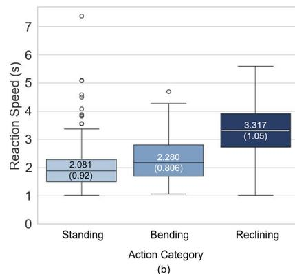
**Figure 10: (a) The comparison of track losing rates (%) of PepperPose, stationary RGB and depth cameras. (b) The reaction speed (second, s) of PepperPose in different action categories. The mean and standard deviation are added to each box.**
