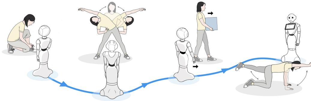
**Figure 1: PepperPose is a companion robot system that optimized to estimate the pose of a user when they move and act diversely in an open space. The magic lies in its ability of actively tracking a person and finding the optimal viewpoint for pose estimation. With PepperPose, the user does not need to wear any devices for accurate action sensing results, and such a capacity opens up new opportunities in embodied interaction and intelligence.**
