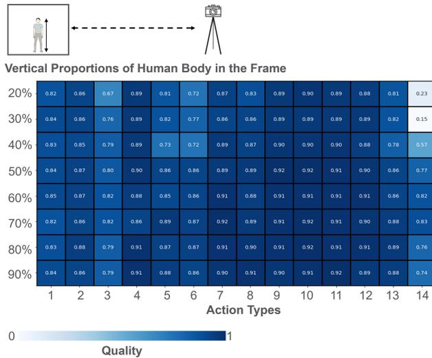
**Figure 3: The results of analyzing the impact of distances between the camera and the user. We test the distances that result in different vertical proportions of a standing-up human in the captured frame, ranging from 90% to 20%. The optimal view angle for each action is used. The action types are denoted by numbers, as shown in Figure 2.**
