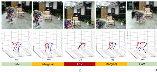
**Figure 11: A visualization of PepperPose’s captured sequence of a user who suddenly changed from standing to bending, approaching the marginal of captured frames (b and d), and eventually the track is lost (c).**
