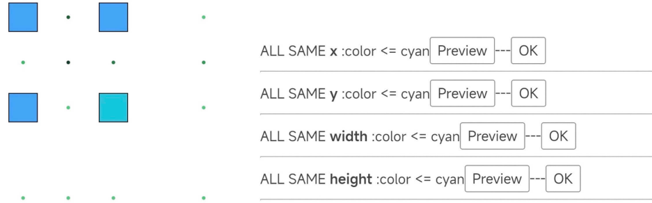
Figure 9: Pre-command prompts in SGDiag. (left) Predicted positions (green dots) for the next element. (right) Predicted subsequent interactions. The last operation is to set the rectangle in the lower right corner to cyan.
