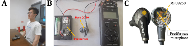
Figure 1: Hardware platform for data collection A: Participant wearing the collection devices B: Three components of the hardware platform C: internal structure of modified Bose QC 20, we embedded the IMU sensor named MPU9250 into the earbuds.
