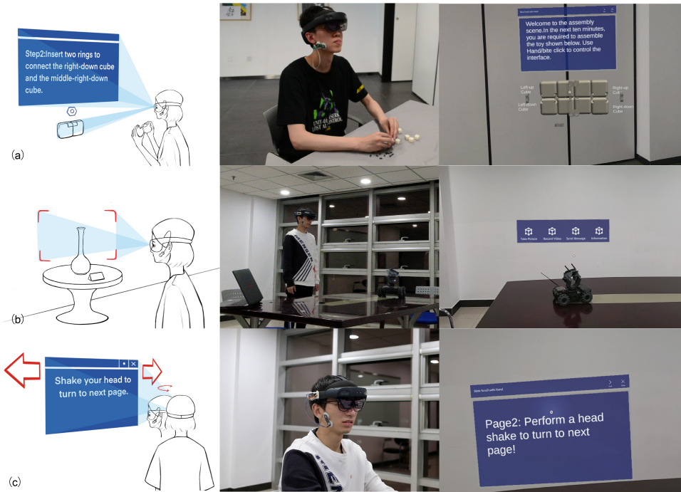
Fig. 10. ClenchClick application scenarios. (a) hands-free requirements: industrial assembly (b) social-friendly interaction: taking pictures (c) gestures beyond selection: clench activated head gesture input
