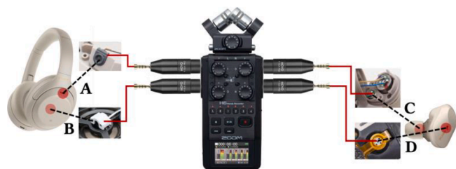
Fig. 4. The hardware setup and the location illustration of the four ANC microphones. This figure was recreated using product pictures from official website and 52Audio.
